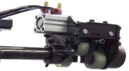
**Bushing Blocks** Optional bushing blocks replace rollers on outboard steady rest when running shaped stock.
