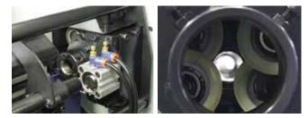
The second roller steady rest is outboard mounted onto the rear of the sliding headstock following the stock as the headstock moves on the z-axis. The bar stock and bar pusher are held in center at the rear of the headstock in both feeding and turning operations.
